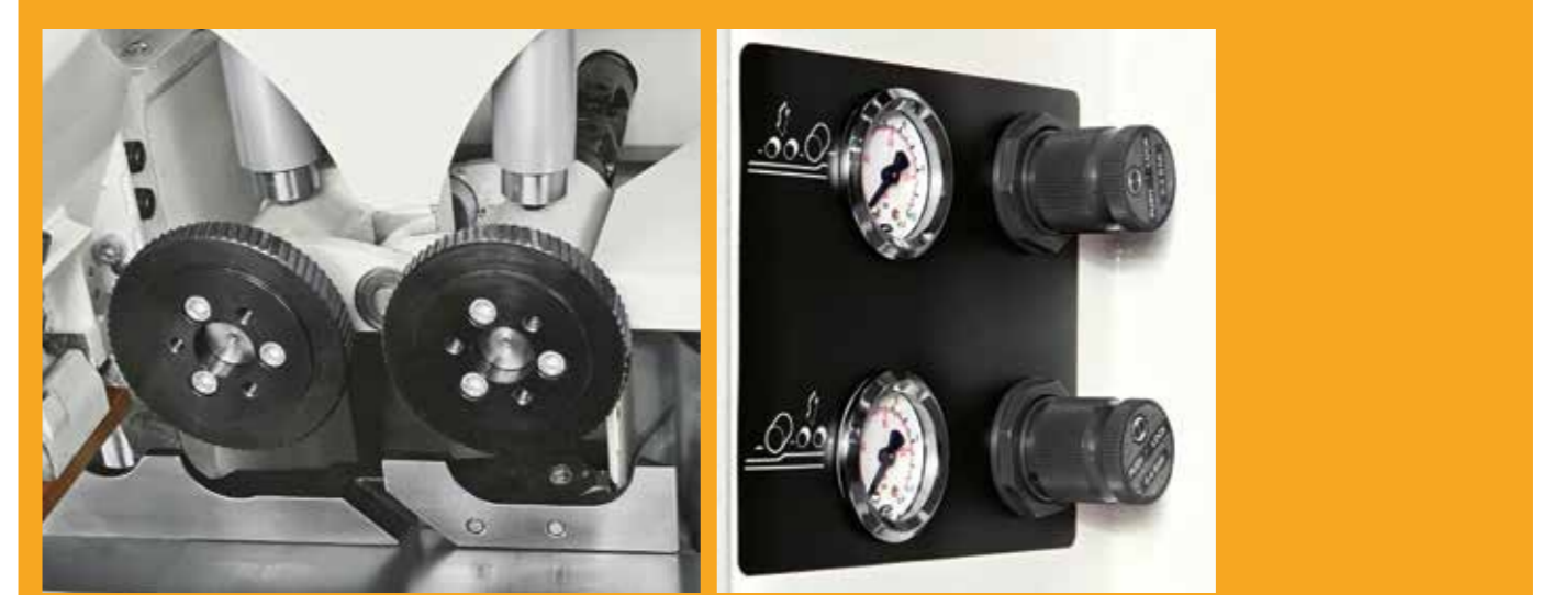
Pneumatic pressure system for the feed rollers. The air pressure can be independently adjusted for the toothed rollers and for the rubber rollers.
